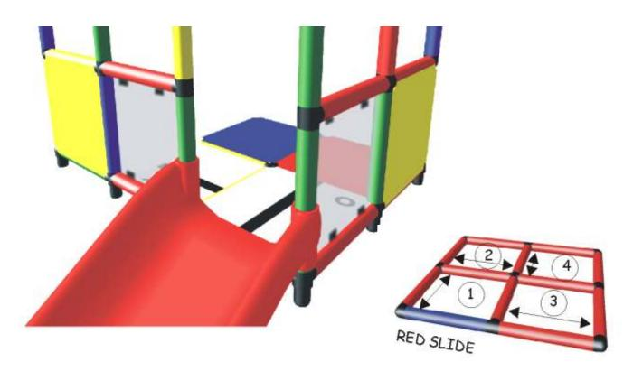
Proper panel alignment is important to install Red Slide
