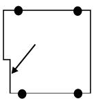
Plexi for red slide Notched plexi panels are required on both sides of the red slide
